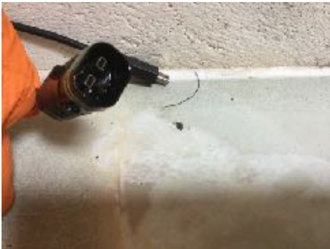
Above: Photos showing silt build up, also moisture ingress in the main battery to motor plug and drain hole still blocked even after cleaning.
