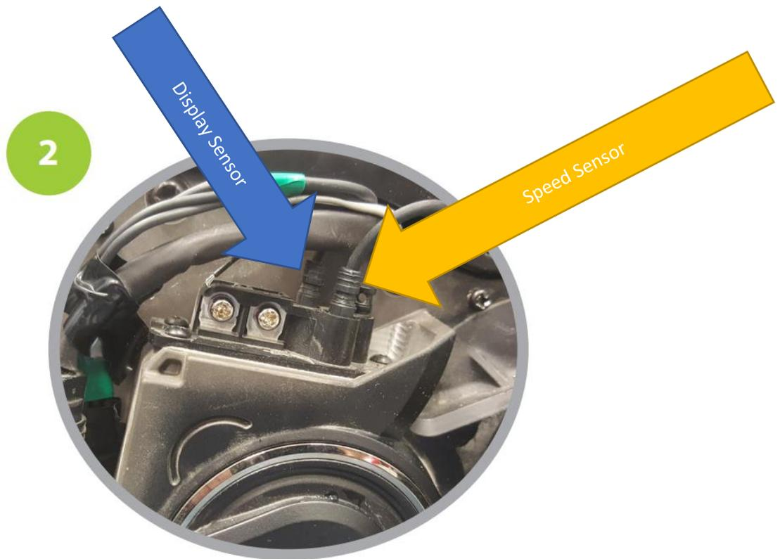
Once removed the protective cap, locate the connector in the foreground among the
