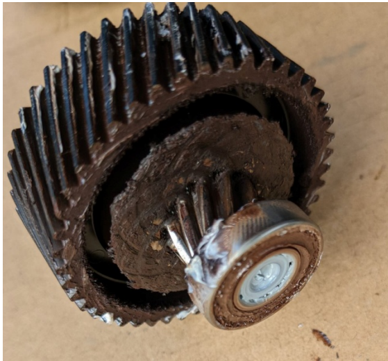
Sprocket with degraded grease transformed in gum:
