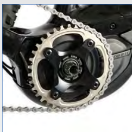
Chainwheel with 8-notch locknut on a SyncDrive Pro Motor
