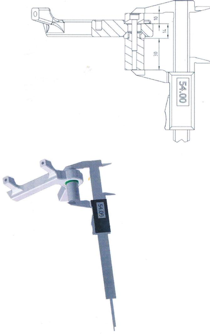
The measurement cylinder must always be positioned against the outer dropout face / the measurement bolt must always be positioned against the inside dropout face. Place the Syntace A12 Conical spacer (green) over the measurement cylinder. Then press the measurement cylinder (with green conical spacer) against the outer face of the dropout and thread the measurement bolt into it by hand.
