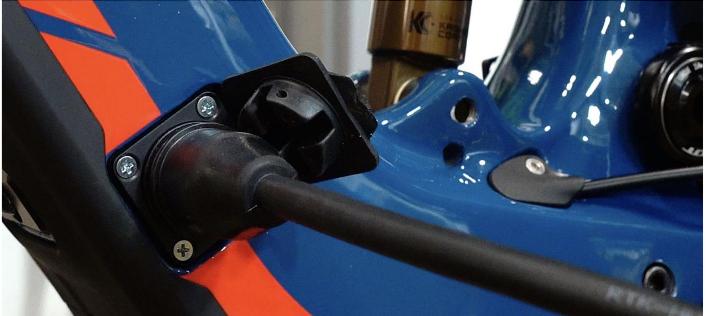
Disconnect the battery from the charging port. Then connect the charging port and battery back to the motor connections and turn the ring control on to test that the system is functioning before replacing the wires into the frame.
