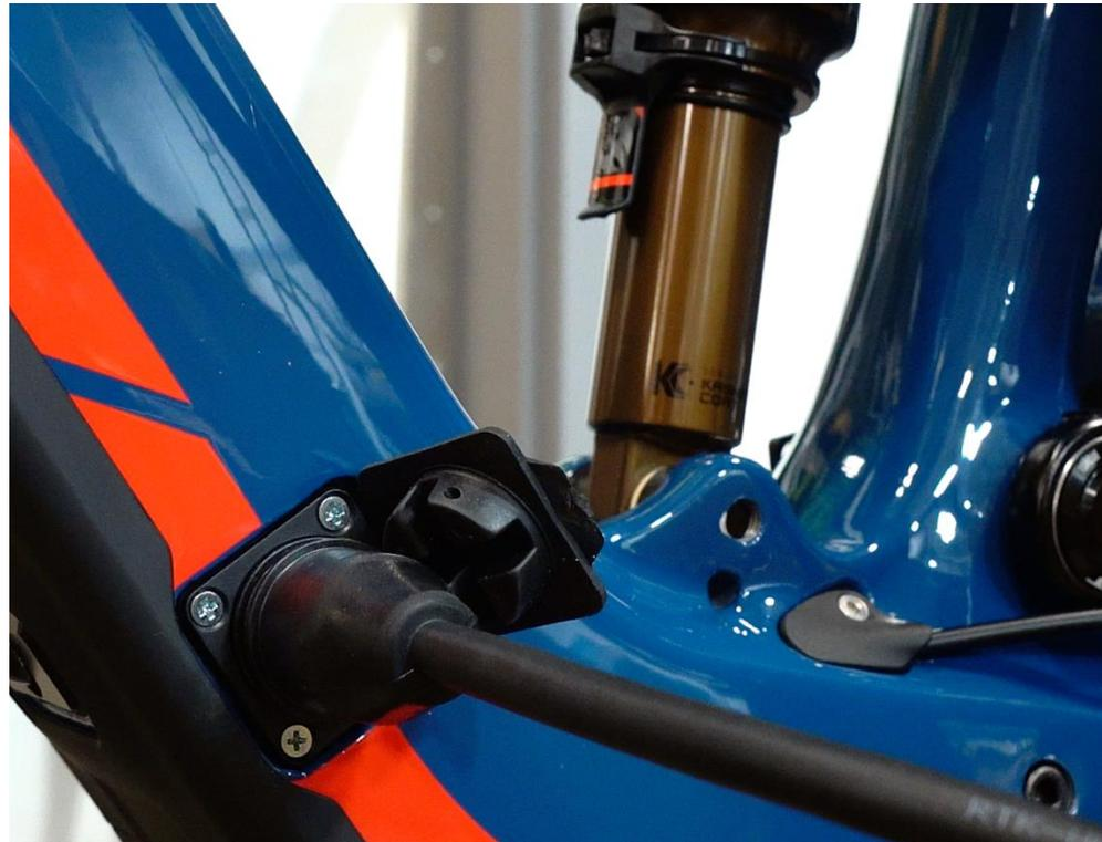
Remove the 4 bolts holding the skid plate on (T25)
