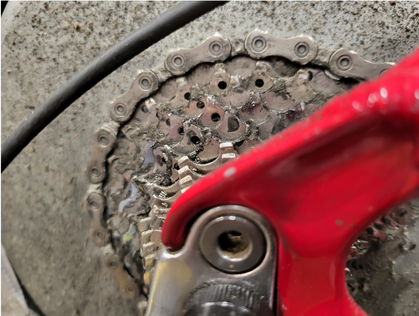
Flower Power post extreme contamination block – 6000km into test
