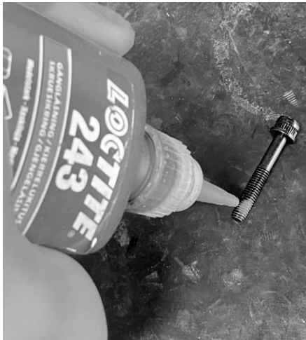
7.1: Apply Loctite 243 to bolts.
