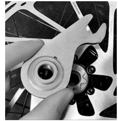
3.5: Remove the torque arm and match cap.
