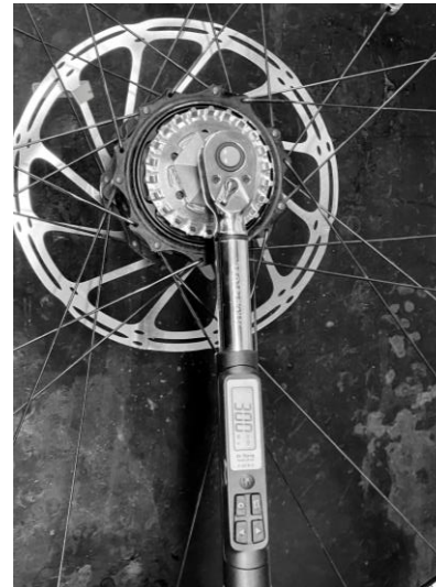
5.3: Torque the locking to 30 Nm.
