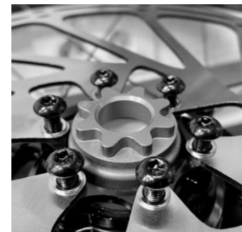
2.2b: Install the rotor bolts with the supplied bolts as shown .
