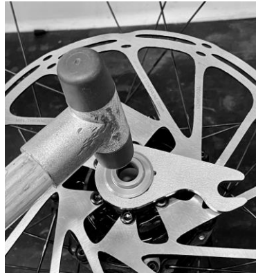
3.3: Gently tap the match cap in place with a rubber mallet.
