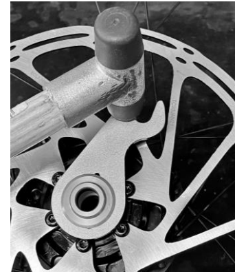
3.4: Gently tap the end of the torque arm with a rubber mallet.
