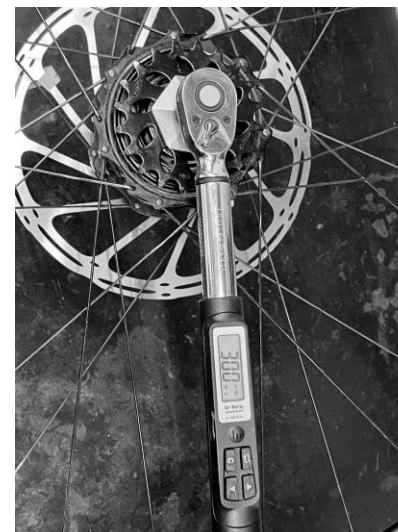
4.3: Torque the locking to 30 Nm.
