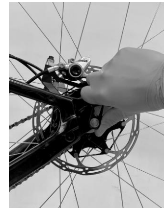
9.5: Tighten the thru-axle according to frame manufacturer specifications.
