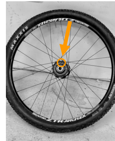
11.4: Turn the wheel around with the oil plug facing upwards .
