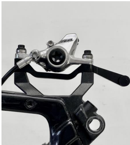
7.2: Install the torque retainer with bolts and conical washers as shown.
