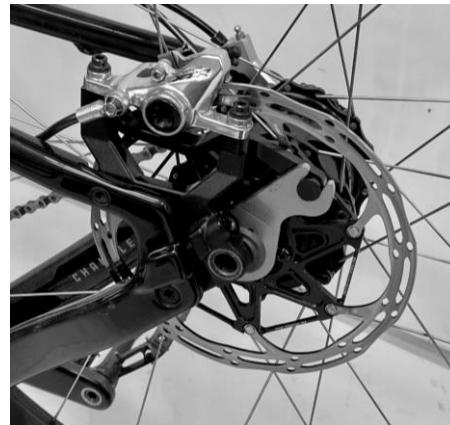
9.3: Align the torque arm and insert the wheel into frame.
