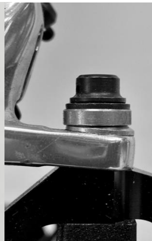
7.2: Install the torque retainer with bolts and conical washers as shown.
