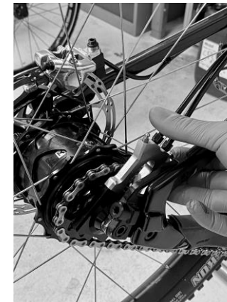
9.4: Install, but do not tighten the thru-axle. Position the actuator in the desired position.
