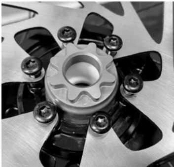
2.1a: Install the brake rotor according to manufacturer specifications.
