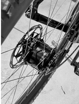
9.1: Install the chain/belt on the gearhub sprocket.
