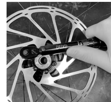
2.3b: Tighten the bolts to 6 Nm in a star pattern.
