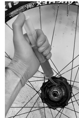
11.5: Refill the gearhub with 20 ml of Kindernay Velvet Fluid.
