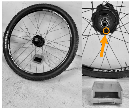
11.3: Position the wheel against the wall at a 45° angle, with the oil plug facing downwards . Let the oil drain for 1-2 hours or more in room temperature.
