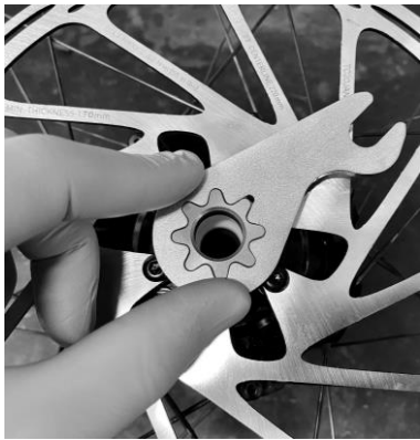
3.1: Install the torque arm.
