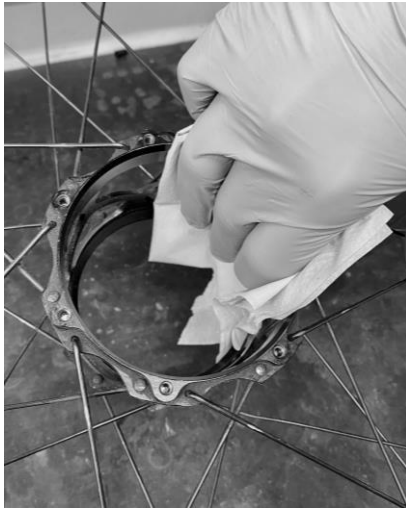
1.1: Clean the SWAP-shell and gearhub housing.
