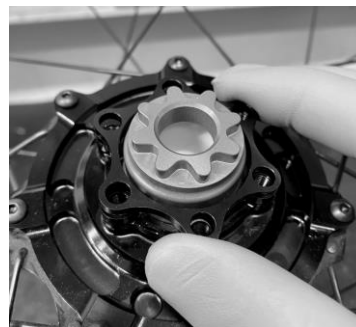
2.1b: Align the 3 mm boost adapter.
