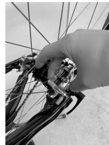
7.3: Install the hub and align the brake caliper.
