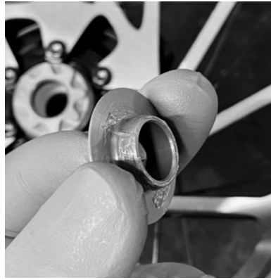
3.2: Lightly grease the end cap press fit surface.
