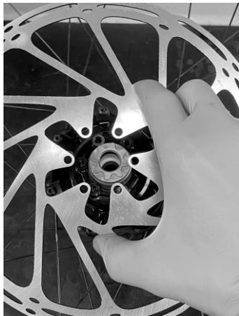
11.1: Remove the torque arm, brake rotor, and sprocket.
