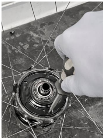
11.2: Unscrew the oil screw on the driveside of the hub.
