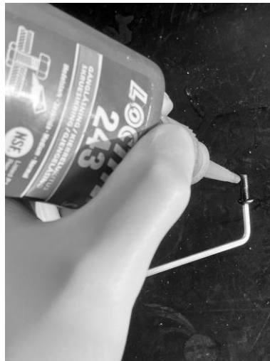
1.2: Apply Loctite 243 to the supplied M4 12 mm bolts
