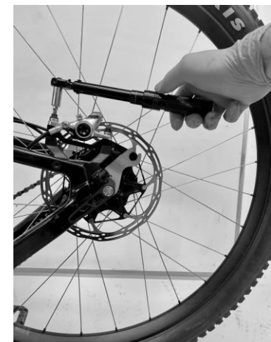
7.4: Torque the PM bolts to 9 Nm.
