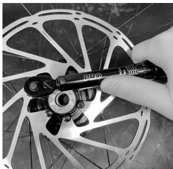
2.2a: Tighten the bolts to 6 Nm in a star pattern.
