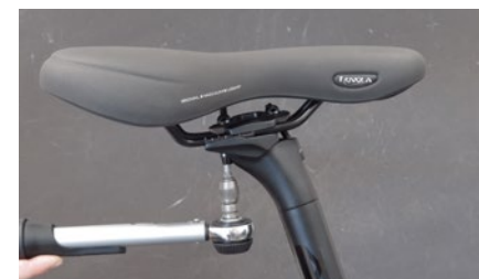
For 1. Loosen screws
