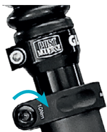
For 3. Tighten the saddle clamp bolt(s)
