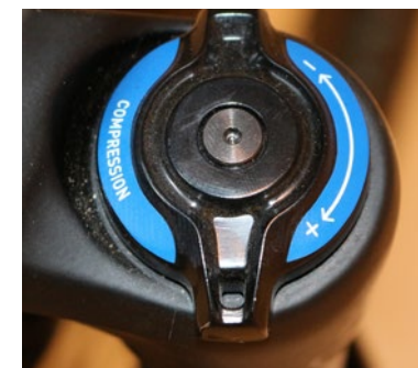
Adjust the compression rate
