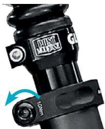
For 1. Loosen the saddle clamp bolt(s)
