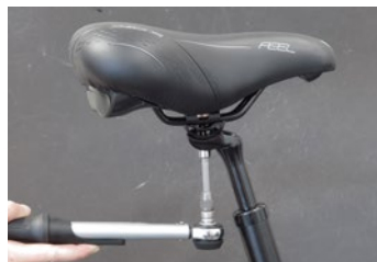
For 1. Loosen the clamping screw
