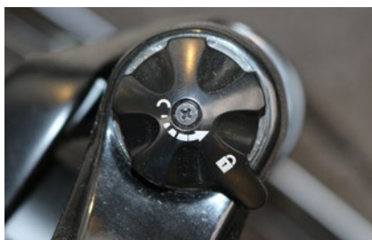
Locking the suspension
