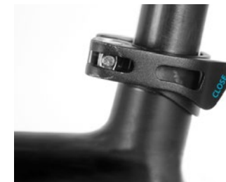
For 2. Quick-release lever closed
