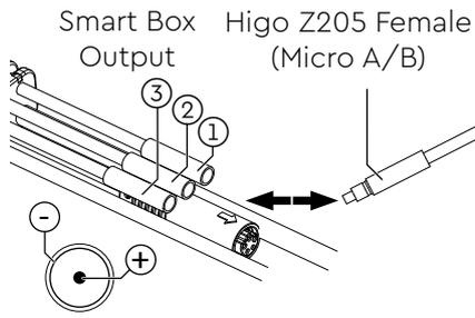
For example, connect the lighting to Output 2 or Output 3 on the Smart Box via compatible Higo Z205 Micro Female connectors. Output 1 is not short-circuit proof.
