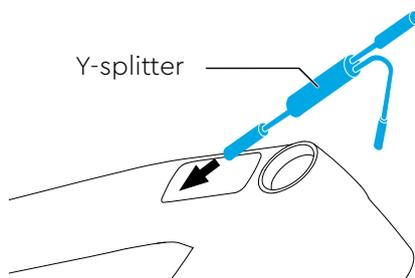
Insert the Y-splitter into the display pocket. First insert the cables into the display pocket.
