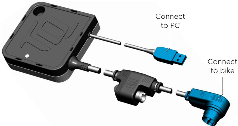
Connect the Dealer Service Tool to the PC via USB port and to the bike via the charging port.
