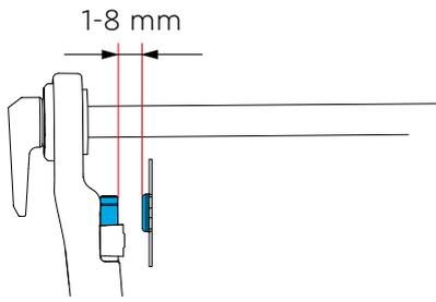
Check the air gap between the speed sensor and magnet. This must be 1-8 mm.
