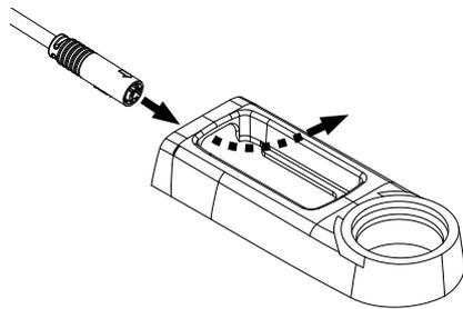
Feed the connection cable for the display / Y-splitter cleanly through the display pocket in the frame.
