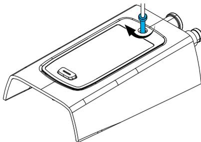
Tighten the included M3x20 display screw with a torque of 0.5 Nm.
