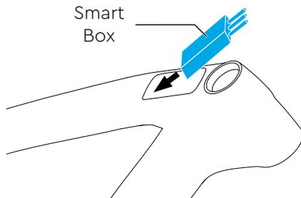
Insert the Smart Box into the display enclosure. To do so, first insert the cables into the display enclosure.
