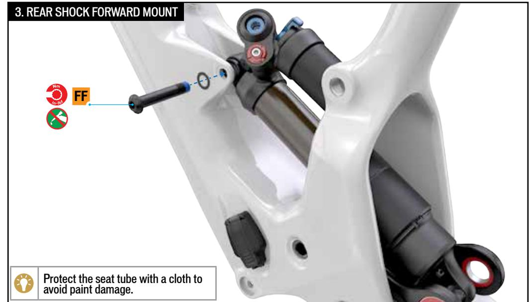
**💡** Protect the seat tube with a cloth to avoid paint damage.
