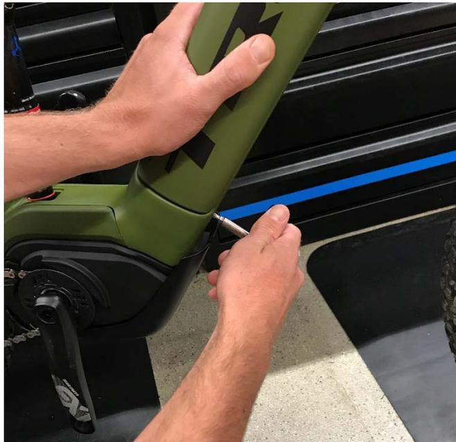
7. Take out the battery to make sure the lock functions properly.
